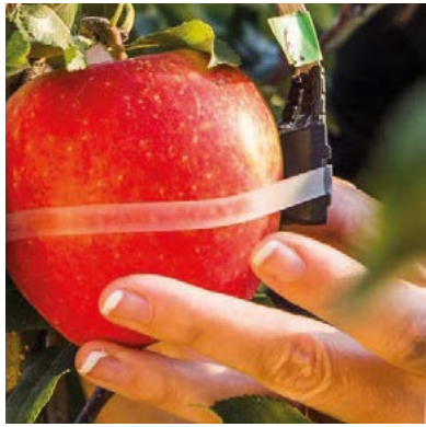
Fig. 1. Set-up of fruit sensor and normalized difference vegetation index (NDVI) of apple fruit measured by means of non-destructive, continuous measurements at the tree over time in days after full bloom (dafb).
